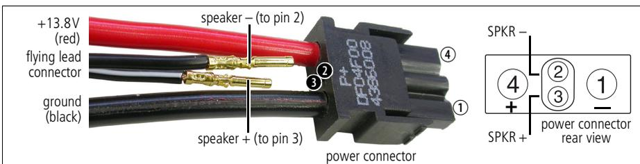
To connect the remote speaker, plug the flying lead into the housing socket. To disconnect the speaker, release the locking mechanism and unplug the flying lead.
